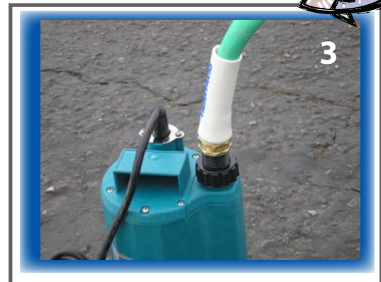
Step 3. Place the pump on the low side of the drain cover where the water will collect. Once water starts to pool check to be sure the pump is in the water. Attach garden hose to pump (at black adapter location). A “snug” fit will do...forcing it more than this may strip the adapter and cause it to leak. NOTE: Attach the end with the swivel for easier turning.
